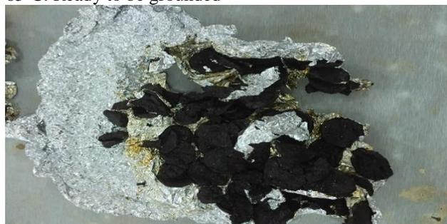
Fig. 7. Dried Banana (China sample) on an aluminium foil ready to be grounded.
