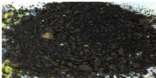
Fig. 5. Banana (Ghana sample) reacted with carbide and allowed to ripen then kept in an oven for 7 days at 65°C, grounded and ready to be sieved.
