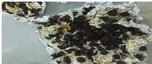
6. Dried Banana (Ghana sample) kept on an aluminium foil at 65°C. Ready to be grounded
